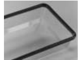
One piece injected molded lens is 1/8" thick DR acrylic.
